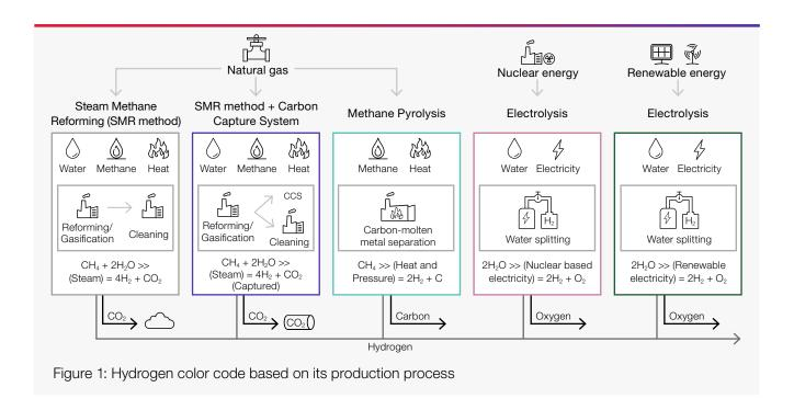
Grey hydrogen is produced using natural gas. The vast majority of hydrogen is grey at the moment<sup>5</sup>. The most common production method used is the Steam Methane Reforming (SMR) method<sup>6</sup>. In this process, methane (CH<sub>4</sub>) reacts with high-temperature steam to produce hydrogen and release CO<sub>2</sub>. The resulting CO<sub>2</sub> emissions are not captured.
