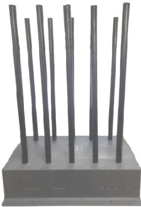
An example 100w jammer legal to buy, but illegal to use in the UK (at time of print) able to impact GNSS and communication spectrum over wide areas impacting safety of operations
