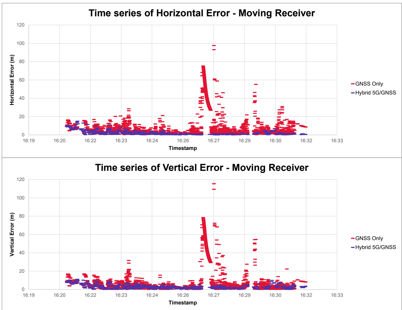
Figure 12: Factory Test Results: Navigation Error for Hybrid 5G/GNSS versus Galileo Only
