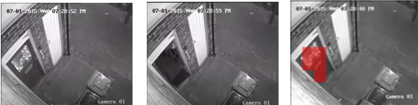
Figure 3 - Example frames of change detection on door opening
